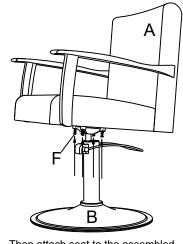
Then attach seat to the assembled bracket and hydraulic.
