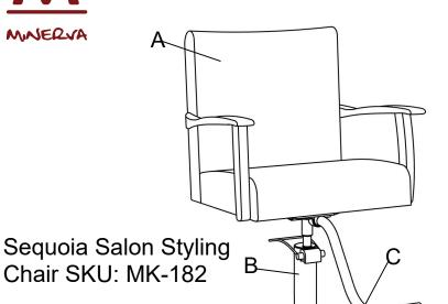
The bracket must be bolted to the hydraulic before the chair can be safely attached. The bracket may already come bolted on the hydraulic, but if not, it must be removed from the chair by removing the four bolts. Now remove the bolt from the piston, place the bracket on the piston, and screw the bolt back into the piston through the bracket.
